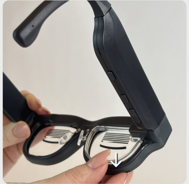
Pressing down on the lens holder
