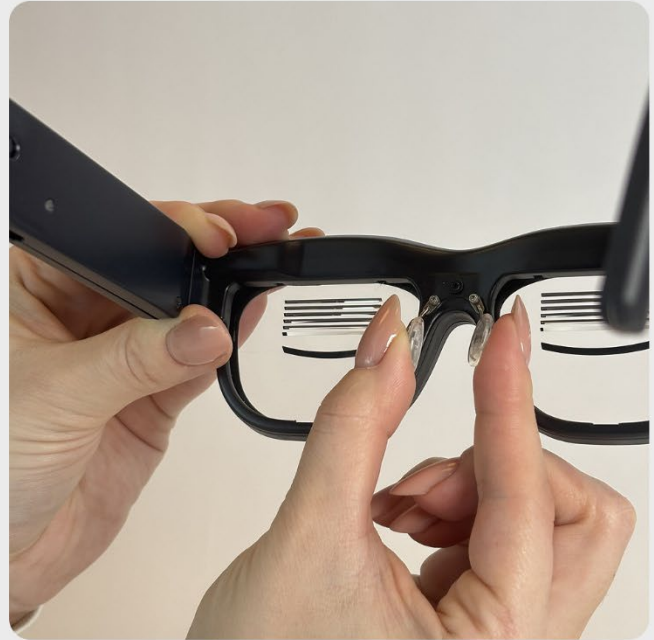
The nose arms have been bent inwards
