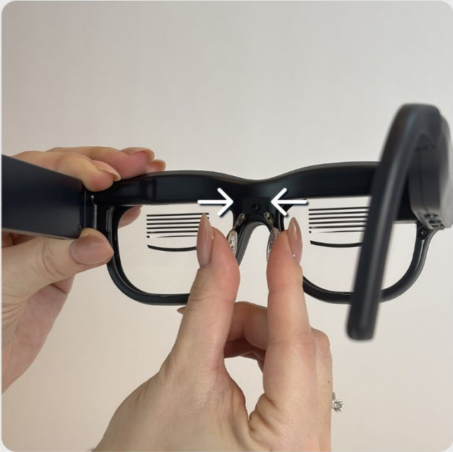
Applying pressure on the nose arms to bend them inwards
